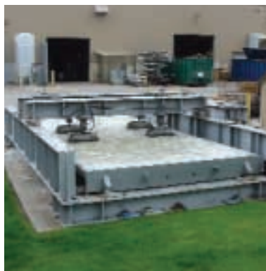
Tandem axle load simulator tests the weighbridge design with millions of weighments.
