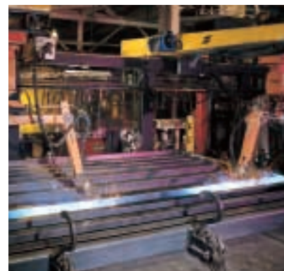
Modules are robotically welded.
