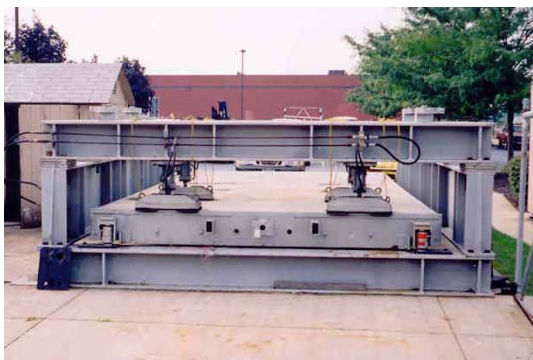
By repositioning the module masher's feet, we can test the strength of a module's end plate.
