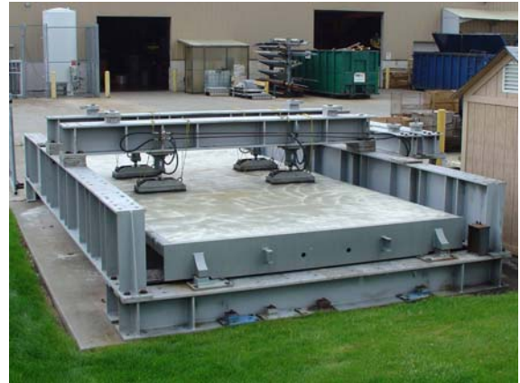
The module masher is used to test the life cycle of a truck scale module.
