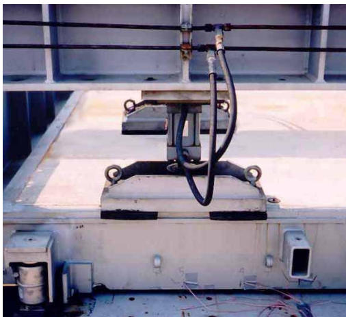
Each foot is equipped with two rubber pads spaced like a pair of tires.
